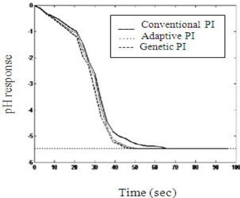
Fig.10. pH response with different control scheme for acidic process.
