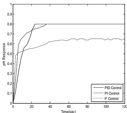
Fig.7. pH response of acidic process with conventional PID control.
