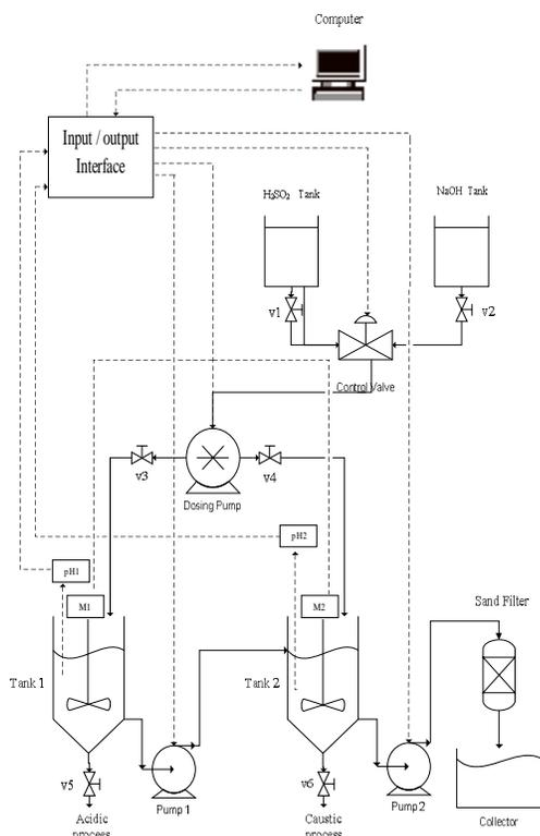
Fig. 3. Schematic diagram of experimental set-up.
