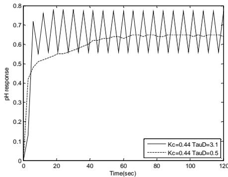
Fig. 9-a: pH response with PD control for hydroxide process.
