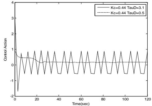
Fig. 9-b. Control action of PD control for hydroxide process.
