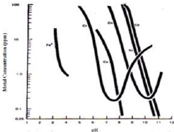
Fig. 1. Precipitation of metals as a function of pH.
