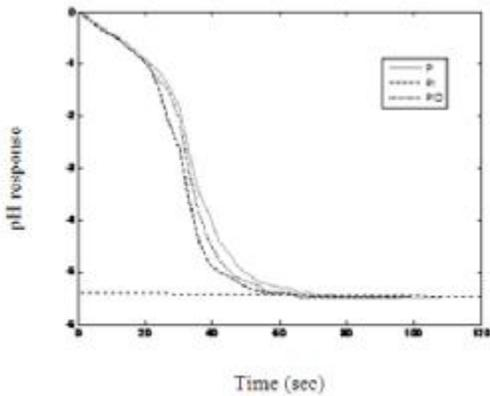
Fig. 8. pH response of hydroxide process with conventional PID control.
