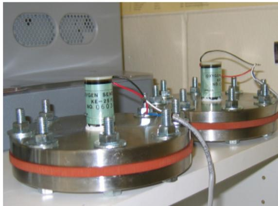
Figure 1 Test set up showing diffusion cells and electrochemical oxygen sensors
