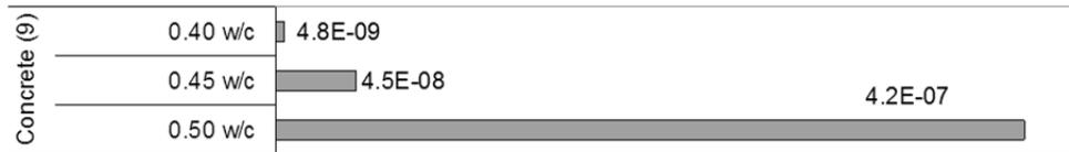
Figure 1. Average oxygen permeation constant for concrete specimens in mol. m<sup>2</sup>/m<sup>3</sup>.atm.sec. [6]
