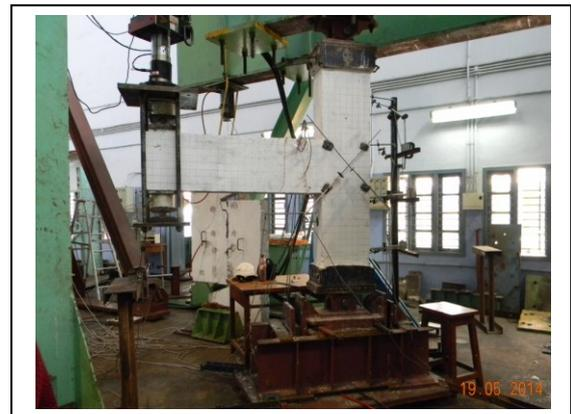
Figure 6. Test set-up arrangement for joints
