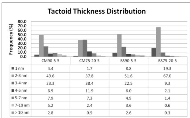
**Figure 4-** Tactoid thickness analysis- TEM results.
