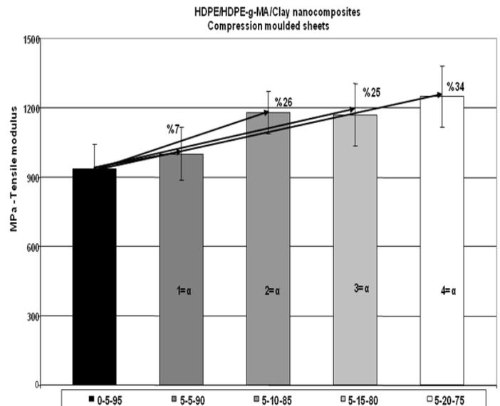
**Figure 6-** Tensile modulus- Compression moulded sheets (15)
