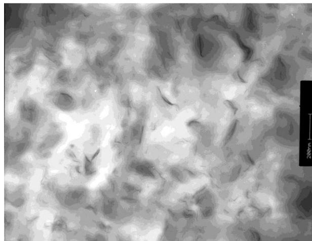
**Figure 2-a** – TEM image of CM sheet –  $\alpha=1$ , scale bar = 200 nm (15)
