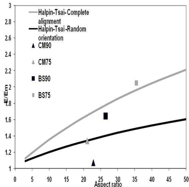
Figure 9 – Experimental relative moduli versus predicted relative moduli
