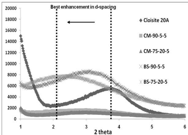
**Figure 1** - XRD traces for Cloisite 20A, Compression moulded sheets (CM) and biaxially stretched sheets (BS) for nanocomposites at  $\alpha = 1$  and  $\alpha = 4$ .
