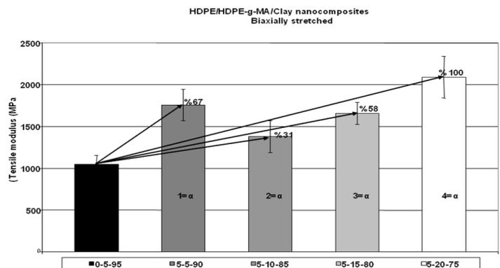
**Figure 7-** Tensile modulus- Biaxially stretched sheets (15)
