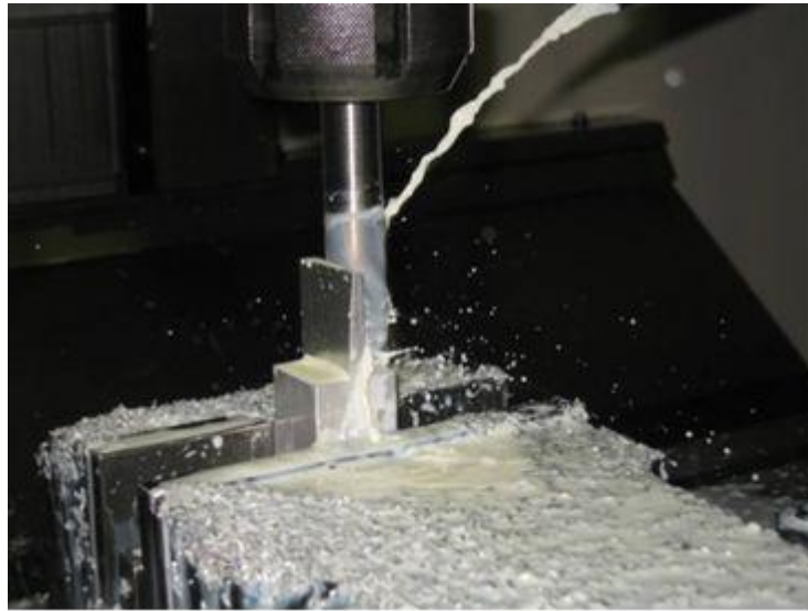
Figure 5: picture of workpiece during rough milling
