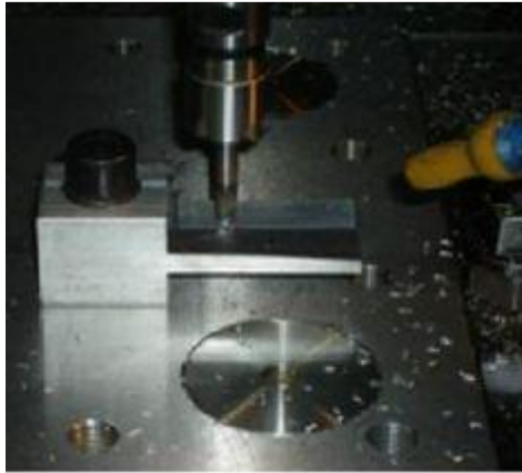
The Longitudinal Outward milling
