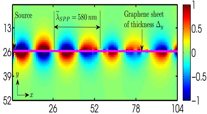
Figure 1: Spatial distribution of  $E_y$  electric field component at time step 20000 showing the SPP surface wave on the Graphene layer.
