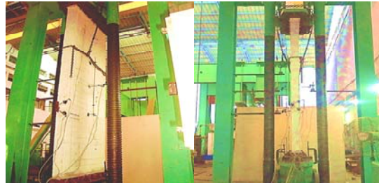
Figure 7. Plain wall panel (a) Schematic diagram (b) Test setup
