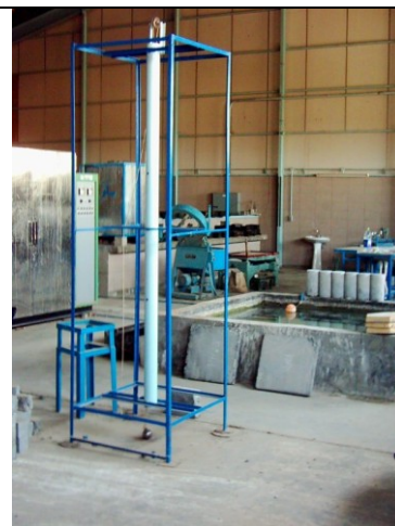
Fig. 2- Rig which is used for low velocity impact test
