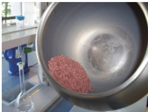
Fig. 4a: ZnO-coated mineral support during the process of drying
