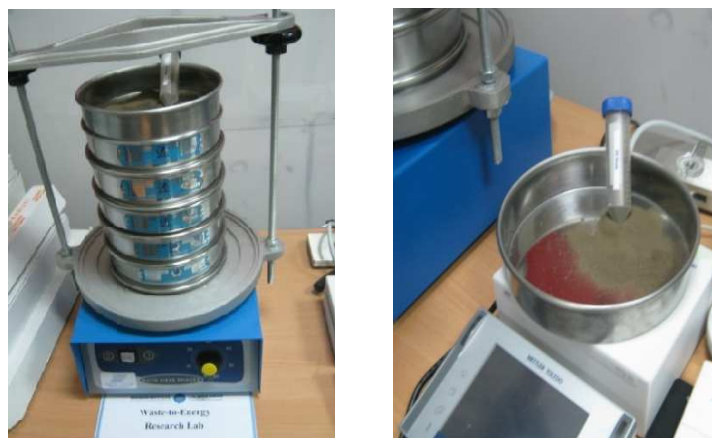
Figure 1: Oil shale sample after milling and during the sieving
