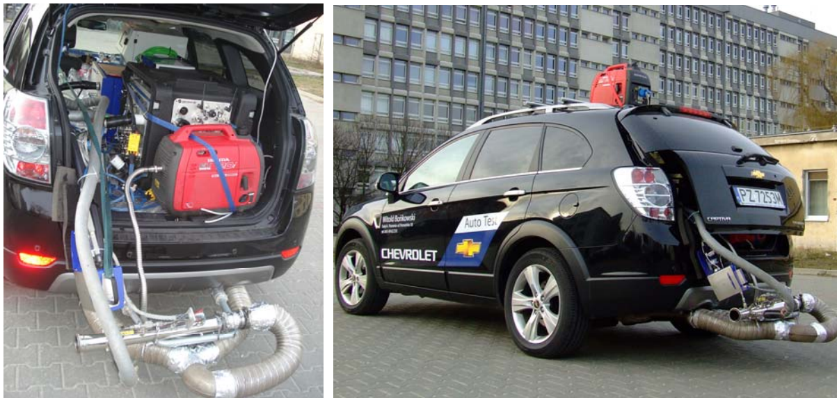
Figure 4. View of SEMTECH DS analyzer fitted in a vehicle
