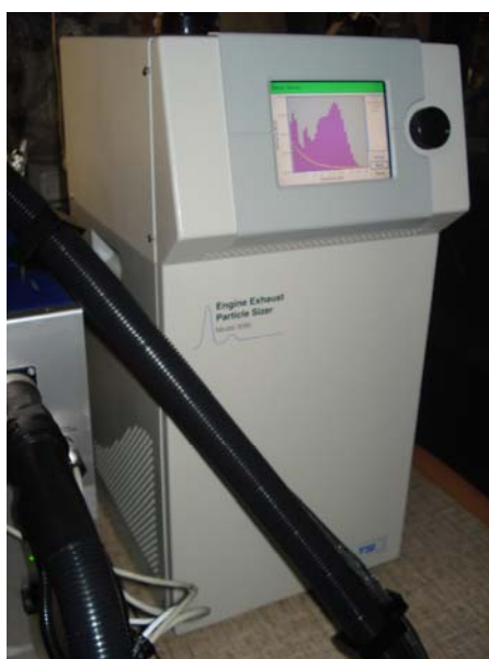
Figure 7. View and schematic diagram of the 3090 EEPS Spectrometer [10]
