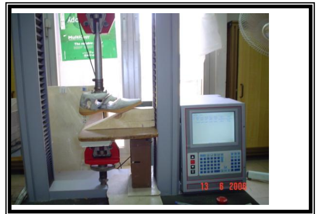
FIGURE (5) DORSIFLEXION AND ENERGY RETURN: A- SACH FOOT B- NEW FOOT
