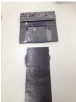
Figure 8: CFRP laminate debonding With 20% IL modified epoxy.
