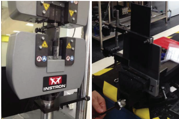
Figure 7: Pull-out test setup of CFRP/steel specimen.
