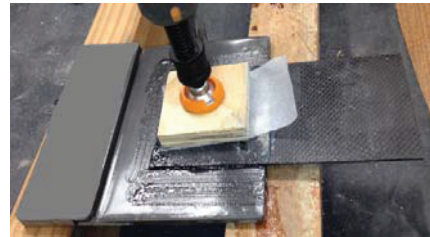
Figure 5: Composite CFRP laminate/steel plate.
