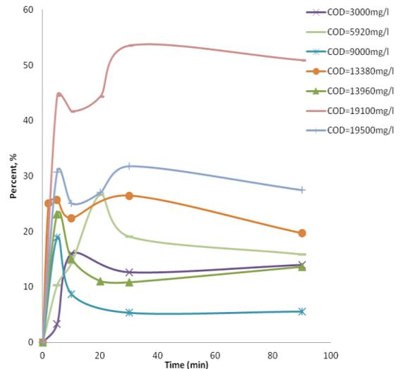
Figure (5.10): Percentage reduction in COD concentration using photo-Fenton's reagent with UV-lamp and air flow at different initial COD.
