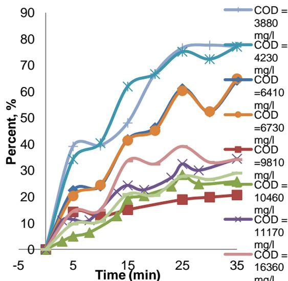
Fig. (5.4): Percentage reduction in COD concentration using Fenton's catalytic process with three dosages at different initial COD concentration.
