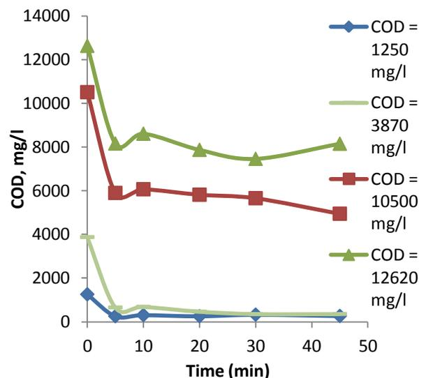
Figure (5.5): Effect of initial COD conc. on COD removal with large dose.
