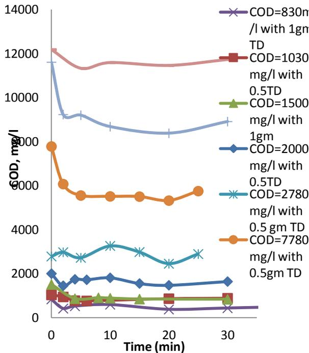
**Figure (5.7): Effect of initial COD concentration on COD removal using Fenton's reagent with titanium dioxide & air.**
