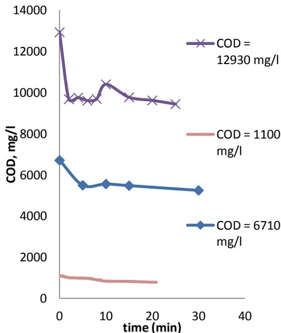
**Figure (5.11):** Effect of initial COD concentration on COD removal using Fenton's reagent with ozone generated from plasma.
