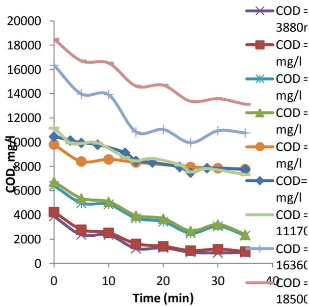
Figure (5.3): Effect of initial COD conc. on COD removal using with three dosages.
