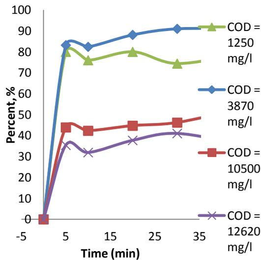
**Fig. (5.6): Percentage reduction in COD concentration using Fenton's catalytic process with large dose at different initial COD concentration.**
