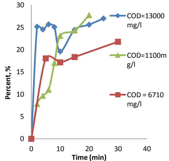
**Figure (5.12):** Percentage reduction in COD concentration using Fenton's reagent with ozone generated from plasma reaction at different initial COD.
