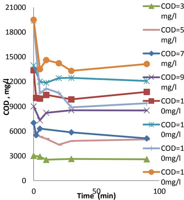
Figure (5.9): Effect of initial COD concentration on COD removal using photo-Fenton's reagent with UV – lamp.
