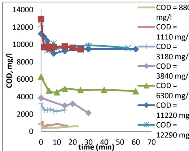
Fig. (5.1): Effect of initial COD conc. by using basic Fenton's process.
