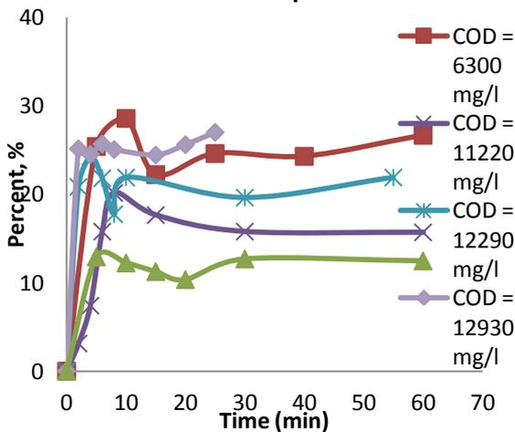
Fig. (5.2): Percentage reduction in COD conc. using basic Fenton's catalytic process at different initial COD concentration.
