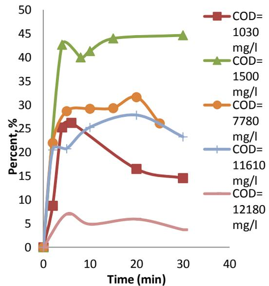
**Figure (5.8): Percentage reduction in COD concentration using Fenton's catalytic process with titanium dioxide and air flow at different initial COD.**
