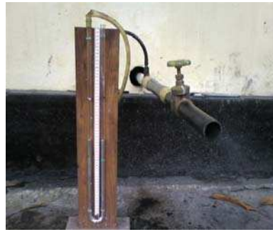
Fig.2: Arrangement of mercury manometer to measure exhaust backpressure.
